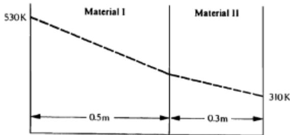
Determine the thermal conductivity of II if the steady-state heat flux is  $12.6 \times 10^3 \text{ W/m}^2 \text{ K}^{-1}$
